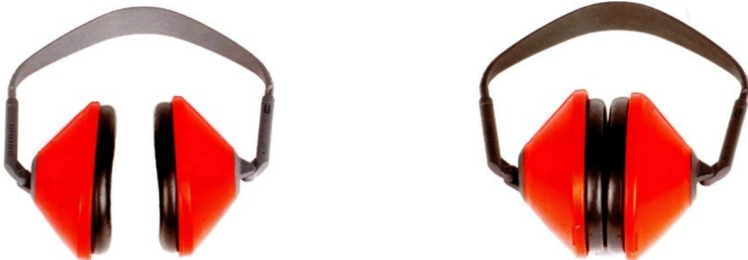
Figure 38 Earmuff headband showing reduced tension (in comparison to tension when new)
