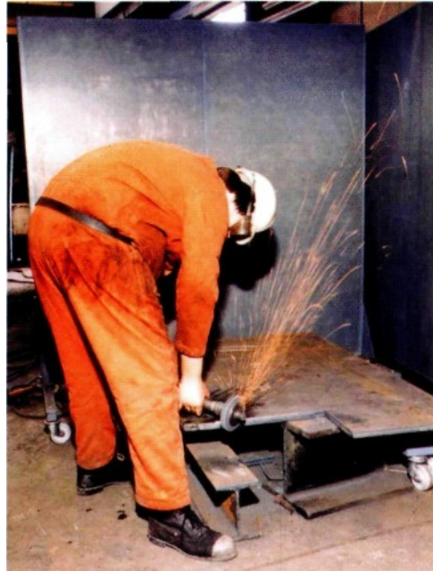
Figure 10 Moveable acoustic screen in an engineering workshop
