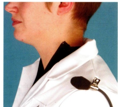
Figure 41 Recommended position for a dosemeter microphone
