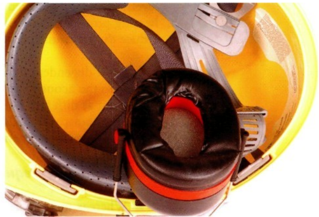
Figure 37 Damaged helmet-mounted earmuff seal due to prolonged storage in 'up' position
