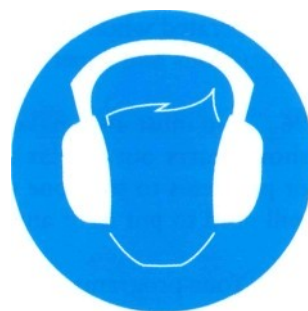
Figure 1 Hearing protection zone sign
