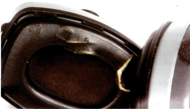
Figure 36 Damaged earmuff seal
